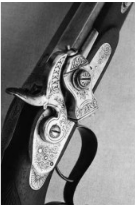
The original lock as designed by rev. Alexander Forsythe. It is generally known as the "Scent bottle lock".
