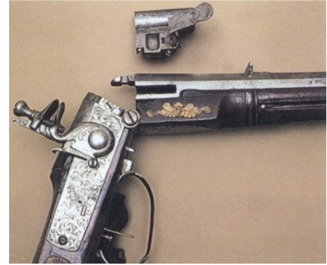
Two breech loading flintlock rifles. The one on the right has removable chambers
