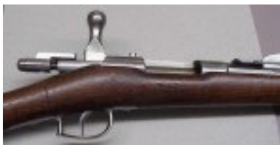
The Dutch Beaumont rifle before and after modification from Beaumont model 71 into Beaumont-Vetterli model 71/88 by the addition of a magazine
