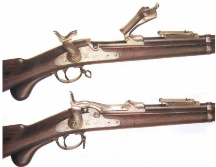
A percussion muzzleloader converted to breechloader: The Springfield Trapdoor rifle
