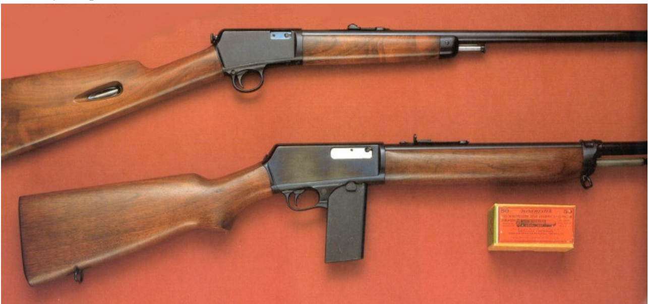
Two firsts for Winchester: on top the model 1903 semiautomatic carbine in calibre .22 long rifle rimfire below the model 1905 semiautomatic carbine in the medium power calibre .32 Winchester centerfire
